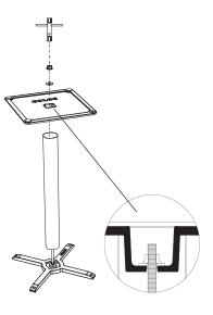
Lay the structure on the ground, making sure that the base and plate are perfectly aligned.
